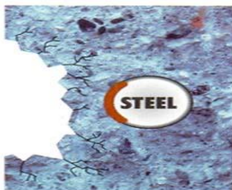
Remove spalled concrete from deteriorating structure.
