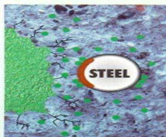
MCI® migrates through concrete without direct application to steel.
