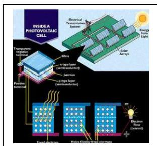
**Photovoltaics (PVs)** are arrays of cells containing a solar photovoltaic material that converts solar radiation into direct current electricity. Materials presently used for photovoltaics include monocrystalline silicon, polycrystalline silicon, amorphous silicon, cadmium telluride, and copper indium selenide/sulfide. Due to the growing demand for renewable energy sources, the manufacture of solar cells and photovoltaic arrays has advanced dramatically in recent years.
