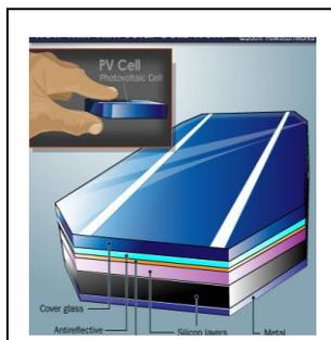
**Fig. The layers of a photovoltaic (PV) solar cell**
